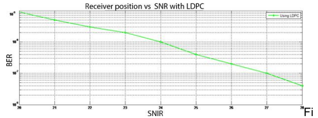
Figure 4.5 represents effects of SNIR and BER using LDPC. Where it indicates the BER reduce in response to the SNIR.
